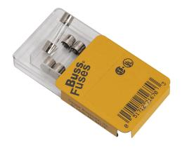
Bussmann fuse, GMA series, small dimension, fast-acting, 2A, 250 VAC, glass tube. Package of 5. Supplemental, electronic protection applications. Manufacturer part number: GMA-2A-R.
