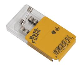
Bussmann fuse, GMA series, small dimension, fast-acting, 15A, 125 VAC, glass tube. Package of 5. Supplemental, electronic protection applications. Manufacturer part number: GMA-15A-R.
