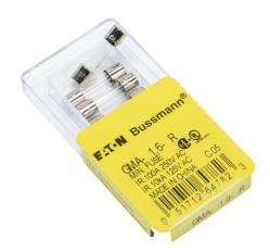
Bussmann fuse, GMA series, small dimension, fast-acting, 1.6A, 250 VAC, glass tube. Package of 5. Supplemental, electronic protection applications. Manufacturer part number: GMA-1.6A-R.
