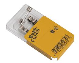
Bussmann fuse, GMA series, small dimension, fast-acting, 1.5A, 250 VAC, glass tube. Package of 5. Supplemental, electronic protection applications. Manufacturer part number: GMA-1.5A-R.
