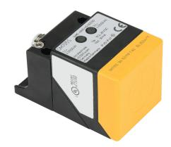
ifm efector inductive proximity sensor, rectangular, 40 x 40 x 66mm body, die-cast zinc housing, PNP, (2) OSSD, 4-20mm enable zone, non-flush, IP65 IP67, 4-pin M12 quick-disconnect.
