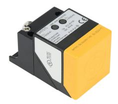
ifm efector inductive proximity sensor, rectangular, 40 x 40 x 66mm body, die-cast zinc housing, PNP, (2) OSSD, 10-15mm enable zone, non-flush, IP65 IP67, 4-pin M12 quick-disconnect.
