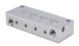
NITRA pneumatic valve manifold, anodized aluminum, rectangular, (4) stations, 1/8in female NPT inlet(s), #10-32 female threaded outlet(s), 1/8in female NPT exhaust(s). For use with GVP-22 and GVP-32 series solenoid valves.
