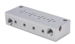
NITRA pneumatic valve manifold, anodized aluminum, white, rectangular, (4) stations, 1/8in female NPT inlet(s), #10-32 female threaded outlet(s), 1/8in female NPT exhaust(s). For use with GVP-22 and GVP-32 series solenoid valves.
