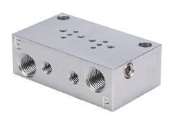
NITRA pneumatic valve manifold, anodized aluminum, white, rectangular, (2) stations, 1/8in female NPT inlet(s), #10-32 female UNF outlet(s), 1/8in female NPT exhaust(s). For use with GVP-22 and GVP-32 series solenoid valves.
