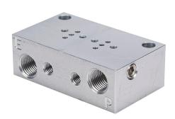
NITRA pneumatic valve manifold, anodized aluminum, rectangular, (2) stations, 1/8in female NPT inlet(s), #10-32 female threaded outlet(s), 1/8in female NPT exhaust(s). For use with GVP-22 and GVP-32 series solenoid valves.
