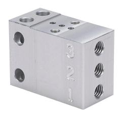
NITRA pneumatic valve manifold, anodized aluminum, white, rectangular, (1) station, #10-32 female UNF inlet(s), #10-32 female UNF outlet(s), #10-32 female threaded exhaust(s). For use with GVP-22 and GVP-32 series solenoid valves.
