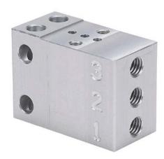
NITRA pneumatic valve manifold, anodized aluminum, rectangular, (1) station, #10-32 female threaded inlet(s), #10-32 female threaded outlet(s), #10-32 female threaded exhaust(s). For use with GVP-22 and GVP-32 series solenoid valves.
