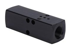
NITRA pneumatic valve manifold, anodized aluminum, black, rectangular, (1) station, 1/8in female NPT inlet(s), 1/8in female NPT outlet(s), vent hole exhaust(s). For use with GVP-22 and GVP-32 series solenoid valves.
