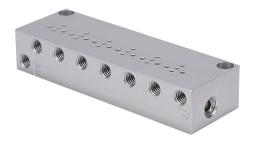
NITRA pneumatic valve manifold, anodized aluminum, white, rectangular, (6) stations, #10-32 female UNF inlet(s), #10-32 female UNF outlet(s), #10-32 female threaded exhaust(s). For use with GVP-21 and GVP-31 series solenoid valves.
