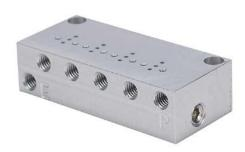
NITRA pneumatic valve manifold, anodized aluminum, rectangular, (4) stations, #10-32 female threaded inlet(s), #10-32 female threaded outlet(s), #10-32 female threaded exhaust(s). For use with GVP-21 and GVP-31 series solenoid valves.
