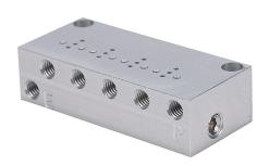
NITRA pneumatic valve manifold, anodized aluminum, white, rectangular, (4) stations, #10-32 female UNF inlet(s), #10-32 female UNF outlet(s), #10-32 female threaded exhaust(s). For use with GVP-21 and GVP-31 series solenoid valves.
