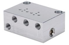
NITRA pneumatic valve manifold, anodized aluminum, white, rectangular, (2) stations, #10-32 female UNF inlet(s), #10-32 female UNF outlet(s), #10-32 female threaded exhaust(s). For use with GVP-21 and GVP-31 series solenoid valves.
