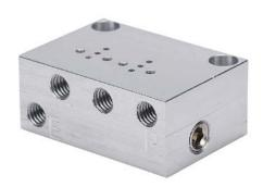
NITRA pneumatic valve manifold, anodized aluminum, rectangular, (2) stations, #10-32 female threaded inlet(s), #10-32 female threaded outlet(s), #10-32 female threaded exhaust(s). For use with GVP-21 and GVP-31 series solenoid valves.
