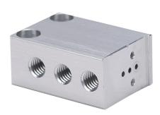
NITRA pneumatic valve manifold, anodized aluminum, white, rectangular, (1) station, #10-32 female UNF inlet(s), #10-32 female UNF outlet(s), #10-32 female threaded exhaust(s). For use with GVP-21 and GVP-31 series solenoid valves.
