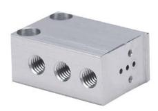
NITRA pneumatic valve manifold, anodized aluminum, rectangular, (1) station, #10-32 female threaded inlet(s), #10-32 female threaded outlet(s), #10-32 female threaded exhaust(s). For use with GVP-21 and GVP-31 series solenoid valves.
