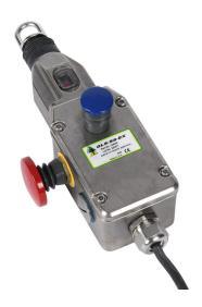
IDEM safety switch, cable-pull interlock, with reset, hazardous location rated, 100m maximum pull cable length, emergency stop, (2) N.C. safety output(s), (2) N.O. monitoring output(s), 316 stainless steel body, pigtail.
