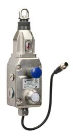
IDEM Z-Range safety switch, cable-pull interlock, 100m maximum pull cable length, emergency stop, (2) OSSD safety output(s), (1) status monitoring output(s), dual color LED, 316 stainless steel body, 8-pin M12 quick-disconnect.
