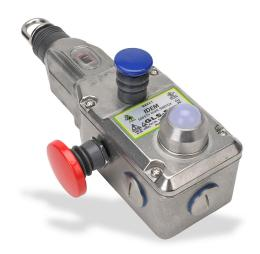
IDEM safety switch, cable-pull interlock, with reset, 100m maximum pull cable length, emergency stop, (3) N.C. safety output(s), (1) N.O. monitoring output(s), 110 VAC LED, 316 stainless steel body, (3) 1/2in NPT cable entries.
