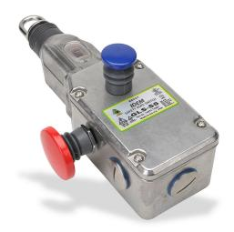
IDEM safety switch, cable-pull interlock, with reset, 100m maximum pull cable length, emergency stop, (3) N.C. safety output(s), (1) N.O. monitoring output(s), 316 stainless steel body, (3) 1/2in NPT cable entries.
