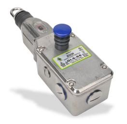
IDEM safety switch, cable-pull interlock, with reset, 100m maximum pull cable length, (2) N.C. safety output(s), (2) N.O. monitoring output(s), 316 stainless steel body, (3) 1/2in NPT cable entries.
