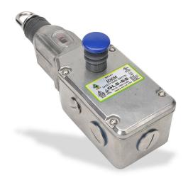
IDEM safety switch, cable-pull interlock, with reset, 100m maximum pull cable length, (3) N.C. safety output(s), (1) N.O. monitoring output(s), 316 stainless steel body, (3) 1/2in NPT cable entries.
