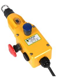
IDEM safety switch, cable-pull interlock, with reset, hazardous location rated, 80m maximum pull cable length, emergency stop, (2) N.C. safety output(s), (2) N.O. monitoring output(s), die-cast aluminum body, pigtail.
