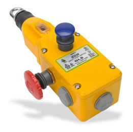
IDEM safety switch, cable-pull interlock, with reset, 80m maximum pull cable length, emergency stop, (3) N.C. safety output(s), (1) N.O. monitoring output(s), die-cast aluminum body, (3) 1/2in NPT cable entries.
