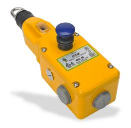
IDEM safety switch, cable-pull interlock, with reset, 80m maximum pull cable length, (3) N.C. safety output(s), (1) N.O. monitoring output(s), die-cast aluminum body, (3) 1/2in NPT cable entries.
