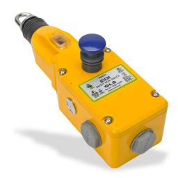
IDEM safety switch, cable-pull interlock, with reset, 80m maximum pull cable length, (2) N.C. safety output(s), (1) N.O. monitoring output(s), die-cast aluminum body, (3) 1/2in NPT cable entries.
