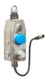
IDEM Z-Range safety switch, cable-pull interlock, 50m maximum pull cable length, emergency stop, (2) OSSD safety output(s), (1) status monitoring output(s), dual color LED, 316 stainless steel body, 8-pin M12 quick-disconnect.
