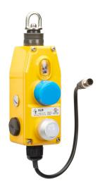
IDEM Z-Range safety switch, cable-pull interlock, 50m maximum pull cable length, emergency stop, (2) OSSD safety output(s), (1) status monitoring output(s), dual color LED, die-cast aluminum body, 8-pin M12 quick-disconnect.
