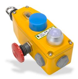
IDEM safety switch, cable-pull interlock, with reset, 50m maximum pull cable length, emergency stop, (3) N.C. safety output(s), (1) N.O. monitoring output(s), 110 VAC LED, die-cast aluminum body, (3) 1/2in NPT cable entries.
