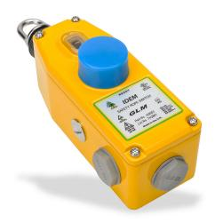
IDEM safety switch, cable-pull interlock, with reset, 50m maximum pull cable length, (2) N.C. safety output(s), (2) N.O. monitoring output(s), die-cast aluminum body, (3) 1/2in NPT cable entries.
