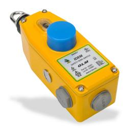
IDEM safety switch, cable-pull interlock, with reset, 50m maximum pull cable length, (3) N.C. safety output(s), (1) N.O. monitoring output(s), die-cast aluminum body, (3) 1/2in NPT cable entries.
