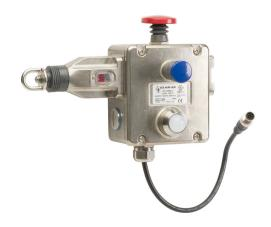
IDEM Z-Range safety switch, cable-pull interlock, 125m maximum pull cable length, emergency stop, right hand head, (2) OSSD safety output(s), (1) status monitoring output(s), dual color LED, 316 stainless steel body, 8-pin M12 quick-disconnect.
