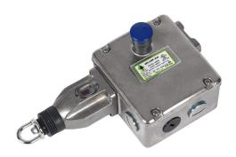
IDEM safety switch, cable-pull interlock, with reset, 125m maximum pull cable length, right hand head, (4) N.C. safety output(s), (2) N.O. monitoring output(s), 316 stainless steel body, (4) 1/2in NPT cable entries.
