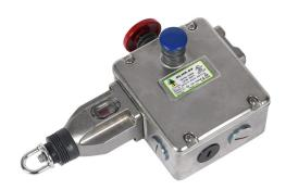
IDEM safety switch, cable-pull interlock, with reset, 125m maximum pull cable length, emergency stop, right hand head, (4) N.C. safety output(s), (2) N.O. monitoring output(s), 316 stainless steel body, (4) 1/2in NPT cable entries.
