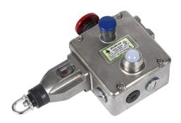
IDEM safety switch, cable-pull interlock, with reset, 125m maximum pull cable length, emergency stop, right hand head, (4) N.C. safety output(s), (2) N.O. monitoring output(s), 110 VAC LED, 316 stainless steel body, (4) 1/2in NPT cable entries.
