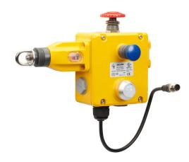
IDEM Z-Range safety switch, cable-pull interlock, 125m maximum pull cable length, emergency stop, right hand head, (2) OSSD safety output(s), (1) status monitoring output(s), dual color LED, die-cast aluminum body, 8-pin M12 quick-disconnect.
