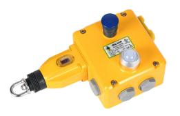
IDEM safety switch, cable-pull interlock, with reset, 125m maximum pull cable length, right hand head, (4) N.C. safety output(s), (2) N.O. monitoring output(s), 110 VAC LED, die-cast aluminum body, (4) 1/2in NPT cable entries.
