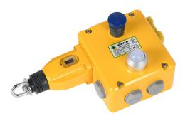
IDEM safety switch, cable-pull interlock, with reset, 125m maximum pull cable length, right hand head, (4) N.C. safety output(s), (2) N.O. monitoring output(s), 24 VDC LED, die-cast aluminum body, (4) 1/2in NPT cable entries.
