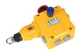
IDEM safety switch, cable-pull interlock, with reset, 125m maximum pull cable length, emergency stop, right hand head, (4) N.C. safety output(s), (2) N.O. monitoring output(s), die-cast aluminum body, (4) 1/2in NPT cable entries.
