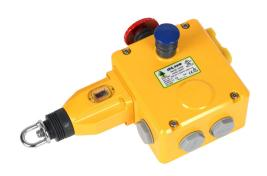
IDEM safety switch, cable-pull interlock, with reset, 125m maximum pull cable length, emergency stop, right hand head, (4) N.C. safety output(s), (2) N.O. monitoring output(s), die-cast aluminum body, (4) 1/2in NPT cable entries.
