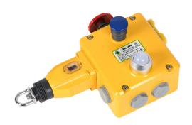
IDEM safety switch, cable-pull interlock, with reset, 125m maximum pull cable length, emergency stop, right hand head, (4) N.C. safety output(s), (2) N.O. monitoring output(s), 110 VAC LED, die-cast aluminum body, (4) 1/2in NPT cable entries.
