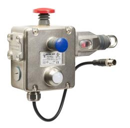
IDEM Z-Range safety switch, cable-pull interlock, 125m maximum pull cable length, emergency stop, left hand head, (2) OSSD safety output(s), (1) status monitoring output(s), dual color LED, 316 stainless steel body, 8-pin M12 quick-disconnect.
