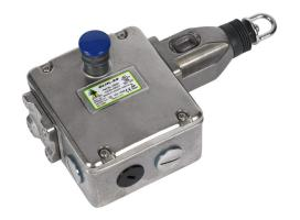
IDEM safety switch, cable-pull interlock, with reset, 125m maximum pull cable length, left hand head, (4) N.C. safety output(s), (2) N.O. monitoring output(s), 316 stainless steel body, (4) 1/2in NPT cable entries.
