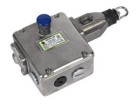
IDEM safety switch, cable-pull interlock, with reset, 125m maximum pull cable length, left hand head, (4) N.C. safety output(s), (2) N.O. monitoring output(s), 316 stainless steel body, (4) 1/2in NPT cable entries.
