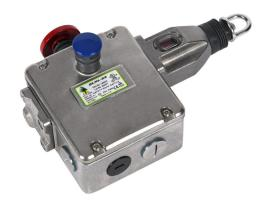
IDEM safety switch, cable-pull interlock, with reset, 125m maximum pull cable length, emergency stop, left hand head, (4) N.C. safety output(s), (2) N.O. monitoring output(s), 316 stainless steel body, (4) 1/2in NPT cable entries.
