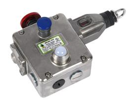
IDEM safety switch, cable-pull interlock, with reset, 125m maximum pull cable length, emergency stop, left hand head, (4) N.C. safety output(s), (2) N.O. monitoring output(s), 110 VAC LED, 316 stainless steel body, (4) 1/2in NPT cable entries.
