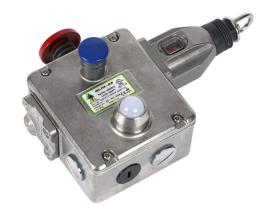
IDEM safety switch, cable-pull interlock, with reset, 125m maximum pull cable length, emergency stop, left hand head, (4) N.C. safety output(s), (2) N.O. monitoring output(s), 24 VDC LED, 316 stainless steel body, (4) 1/2in NPT cable entries.
