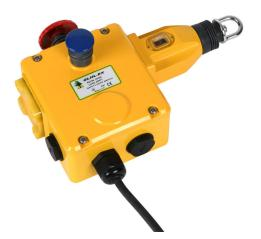
IDEM safety switch, cable-pull interlock, with reset, hazardous location rated, 125m maximum pull cable length, emergency stop, left hand head, (2) N.C. safety output(s), (2) N.O. monitoring output(s), die-cast aluminum body, pigtail.
