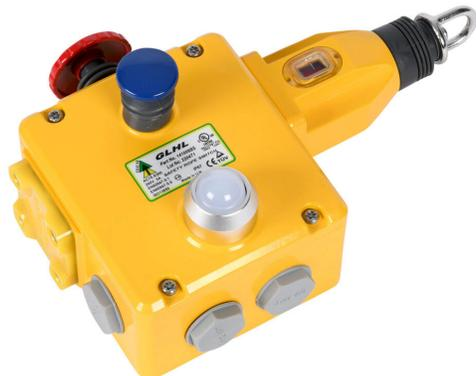
IDEM safety switch, cable-pull interlock, with reset, 125m maximum pull cable length, emergency stop, left hand head, (4) N.C. safety output(s), (2) N.O. monitoring output(s), 110 VAC LED, die-cast aluminum body, (4) 1/2in NPT cable entries.
