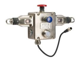
IDEM Z-Range safety switch, cable-pull interlock, 250m maximum pull cable length, emergency stop, dual head, (2) OSSD safety output(s), (1) status monitoring output(s), dual color LED, 316 stainless steel body, 8-pin M12 quick-disconnect.
