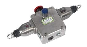
IDEM safety switch, cable-pull interlock, with reset, 250m maximum pull cable length, emergency stop, dual head, (4) N.C. safety output(s), (2) N.O. monitoring output(s), 316 stainless steel body, (4) 1/2in NPT cable entries.
