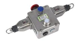
IDEM safety switch, cable-pull interlock, with reset, 250m maximum pull cable length, emergency stop, dual head, (4) N.C. safety output(s), (2) N.O. monitoring output(s), 110 VAC LED, 316 stainless steel body, (4) 1/2in NPT cable entries.
