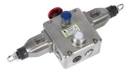
IDEM safety switch, cable-pull interlock, with reset, 250m maximum pull cable length, emergency stop, dual head, (4) N.C. safety output(s), (2) N.O. monitoring output(s), 24 VDC LED, 316 stainless steel body, (4) 1/2in NPT cable entries.
