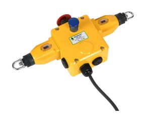
IDEM safety switch, cable-pull interlock, with reset, hazardous location rated, 250m maximum pull cable length, emergency stop, dual head, (2) N.C. safety output(s), (2) N.O. monitoring output(s), die-cast aluminum body, pigtail.
